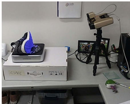
Figure 12: The Complete set-up for the 3D scanner and turn table.
