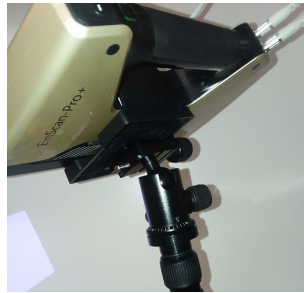
Figure 5: Position the scanner securely into the mount
