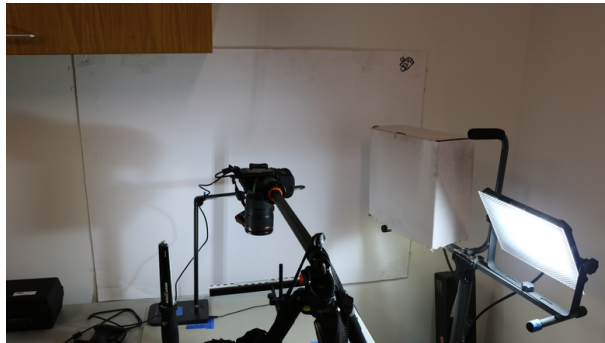
Figure 24: A new lighting system was designed for high resolution photography
