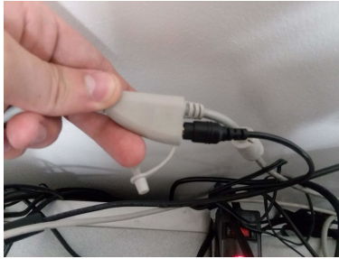
Figure 2: Insert the black power cord into the hub on the USB cord.
