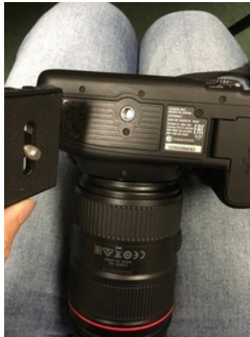
Figure 8: Camera attachment point
