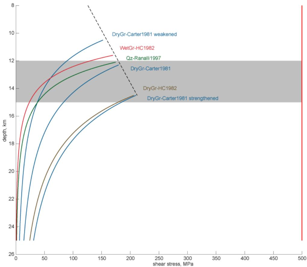
**Figure S1.** Schematic representation of different rheological law considered for the matrix. Dashed line represents the frictional strength of the matrix. Curved lines represent the different viscous strengths for different materials. Gray box shows the estimated depth of the pluton according to de Saint-Blanquat et al. (2001).
